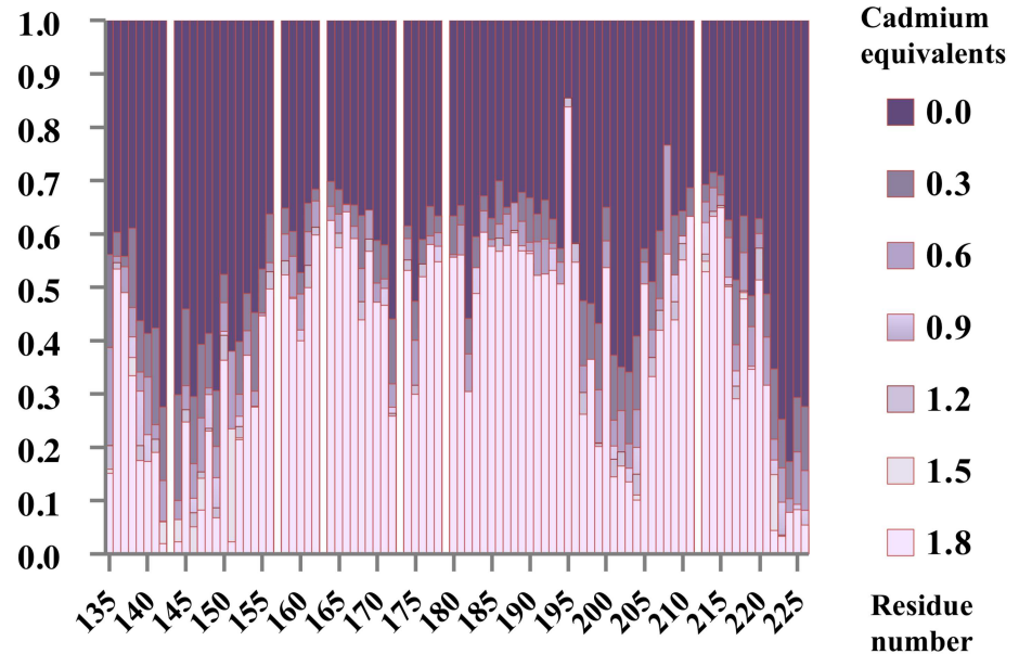
Fig 5. Peak volume evolution of the 1H-15N TROSY with increasing concentrations of CdCl 2 . The cadmium concentration was increased from 0 to 1.8 equivalents. The peak volumes are normalized against the highest peak volume in the TROSY experiment without cadmium. No bar indicates either the presence of proline or a residue (Asn 212 ) that could not be unambiguously identified on the spectrum. Extremely perturbed peaks following cadmium addition identify three principal regions potentially involved in dimerization: Tyr 139 -Gly 151 , Ala 197 -Leu 204 and Leu 221 -Thr 226 .
