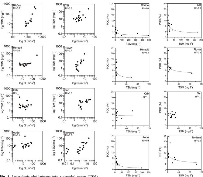
**Fig. 5.** Logarithmic plot between total suspended matter (TSM) concentration and average daily water discharge (Q) with  $R^2$  values obtained using the sediment rating curve:  $TSM = a \times Q^b$ , where a and b are regression coefficients.
