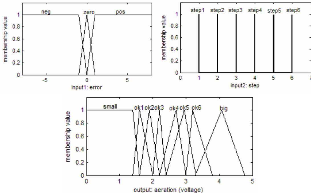
Fig. 5. Fuzzy sets of the on-line DO controller.
